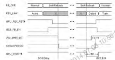
Figure 18-12. GC6 2.0 Entry/Exit Sequence Timing Diagram
